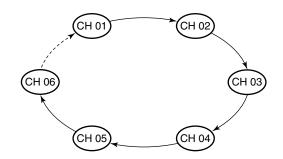
Normal scan, like priority scan, searches through all tag channels in sequence. However, unlike priority scan, Channel 16 is not checked unless Channel 16 is set as a tag channel.
